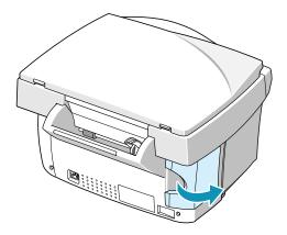
3 Connect the printer cable. Use only USB cable (shipped with your product) or IEEE 1284 compliant parallel cable (purchase separately).
